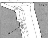
Do not lock the switch "ON" when drilling by hand so that you can instantly release the trigger switch if the bit binds in the hole.
